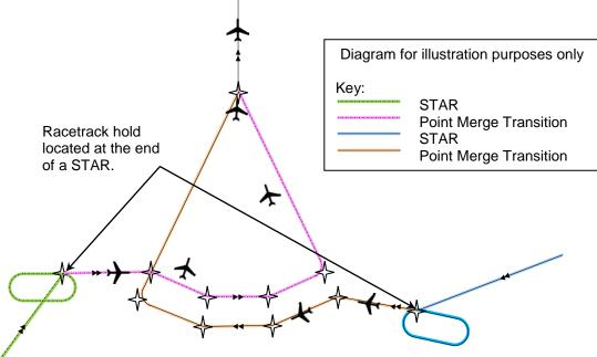
Figure 2 - Point Merge procedure with racetrack holds.
