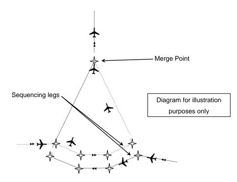
Figure 1 - Point Merge Procedure
